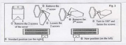
NB: control box should always be under the unit, either on the right or on the left side of the unit.
